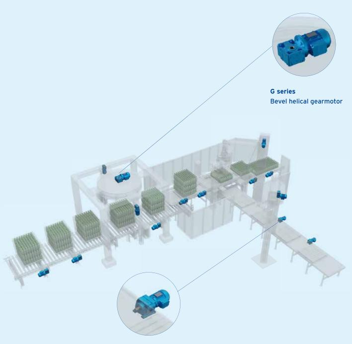
**iFIT series** Helical inline gearmotors
